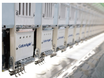
四色高速机头 4-Color High-Speed Machine Head
